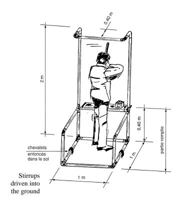
Shooting stand made of coloured P.V.C. tubes, [] 50 mm Straight tubes + interlocking elbows.
